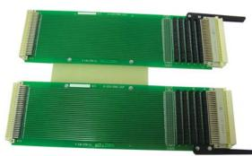
Length: Height: Voltages: Layer Design: 11.75" (298mm) 3U, 3.94" (100mm) or 6U (233.35mm) +5, Aux A & Aux B, GND 8-layer; trace shielding for each signal line
